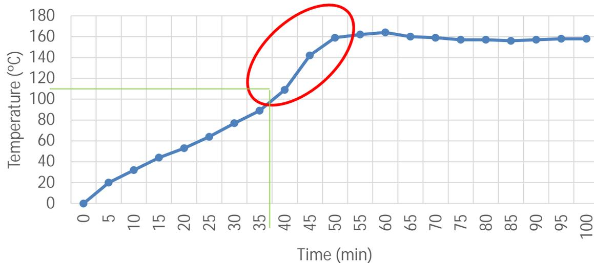
Figure 10 : Temperature profile during hydration process
