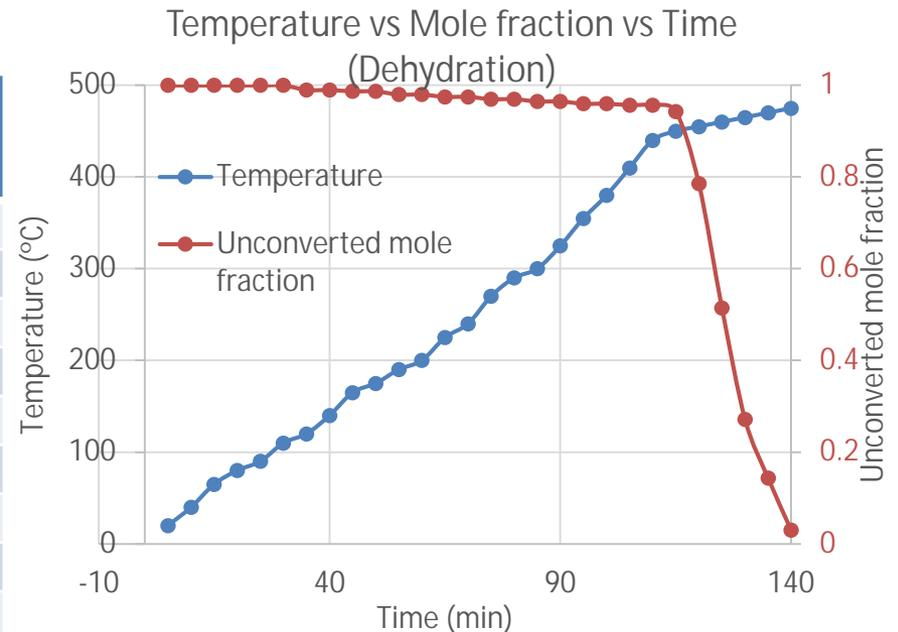
Figure 8 : Temperatures and unconverted mole fraction during dehydration reaction  $P = 3.17 \text{ kPa}$
