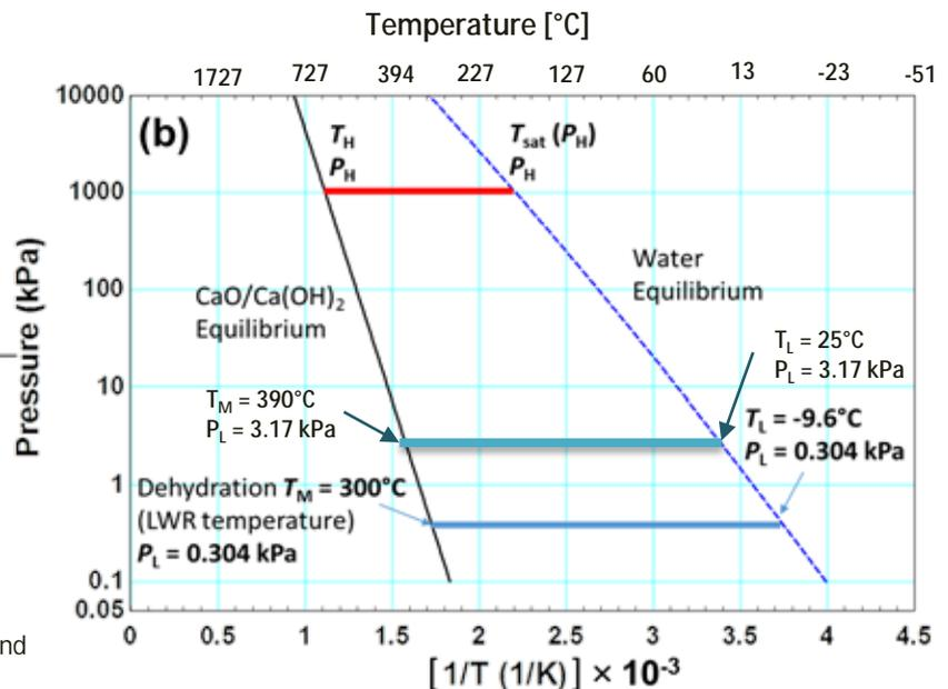
Heat pump cycle on Clausius-Clapeyron diagram showing equilibrium of  $\text{CaO/Ca(OH)}_2$  and  $\text{H}_2\text{O(l)}/\text{H}_2\text{O(g)}$
