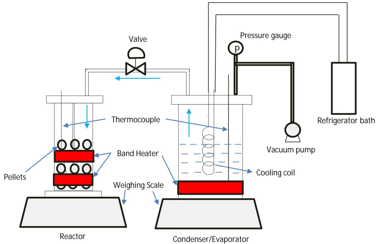
Figure 7 : Schematic of Experimental Setup
