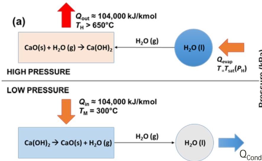
Schematics of component of CHP system
